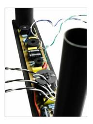
A completely new linear crossover layout, with the copper circuit paths arranged in the direction of electron flow, takes into account the potential for sympathetic and parasitic interactions among crossover components that may inject unwanted noise and distortions while allowing for more direct and efficient transfer of signal to the drivers which leads to a greater level of detail and purity.
